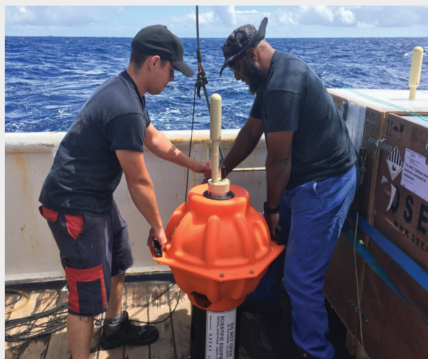
Figure 6. Launch of a MERMAID in the waters around Tahiti. No specialized equipment is needed. Once waterborne, MERMAID is completely autonomous and reports earthquake records via satellite, on average every 6.25 days. Photograph courtesy of Frederik J. Simons.
