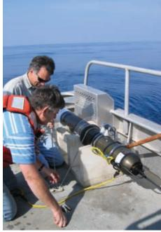
a hydrophone, an off-the-shelf instrument that detects sound waves underwater – effectively, a single-component 'seismometer'. In principle, our MERMAID – Mobile Earthquake Recording in Marine Areas by Independent Divers – was now born.
