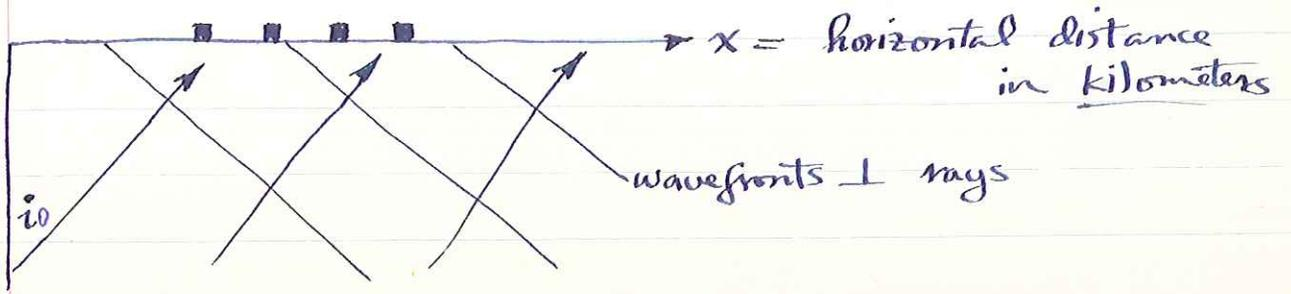
$$p = \frac{a \sin i_0}{v_{crust}} = \frac{dT}{d\Delta} = a \frac{dT}{a d\Delta} = a \frac{dT}{dx}$$
