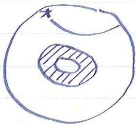
$\alpha(r)$  and  $\beta(r)$  are, except for LVE, increasing fns of depth, so the rays dive down as shown to arrive along least time paths.
