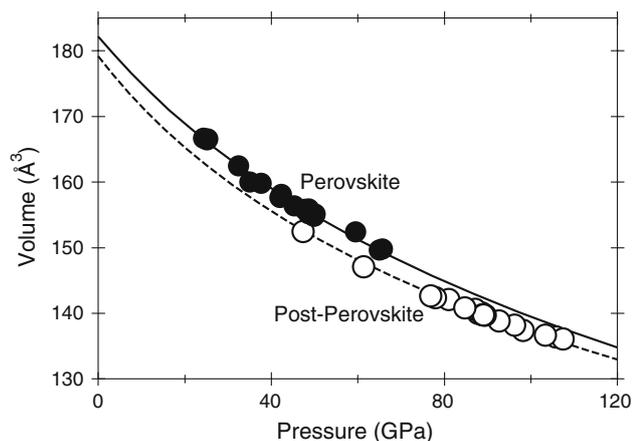
**Fig. 3** Comparison of experimental pressure–volume measurements for MgGeO<sub>3</sub> Pv and pPv phases. *Solid circles* Pv data (this study); *open circles* pPv data (Kubo et al. 2006). *Solid and dashed curves* are fits using third order Birch–Murnaghan EOS for the Pv and pPv studies, respectively. Data below 47 GPa for the pPv phase were not used in the equation of state determination and are not shown (Kubo et al. 2006)
