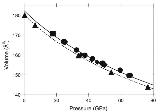
**Fig. 2** Pressure–volume data for MgGeO<sub>3</sub> Pv phase. Solid curve is a fit using third order Birch–Murnaghan EOS. Dashed line is a third order Birch–Murnaghan EOS fit to the theoretical data. Solid circles and diamonds experimental compression and decompression data, respectively; solid triangles theoretical calculations; solid square Leinenweber et al. (1994)
