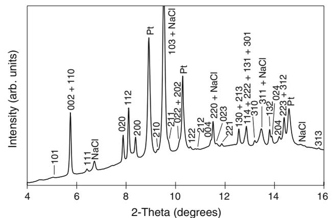
**Fig. 1** Representative X-ray diffraction pattern at 65 GPa during the compression run.  $\text{MgGeO}_3$  Pv peaks are labeled with their respective  $hkl$ . Also indicated are peaks from NaCl (B2 phase) and Pt
