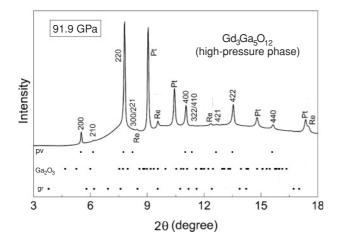
FIG. 1. Angle-dispersive x-ray diffraction pattern (wavelength  $\lambda = 0.3344$  Å) of high-pressure Gd<sub>3</sub>Ga<sub>5</sub>O<sub>12</sub> phase (Pv) indexed to a cubic unit cell. Tick marks show expected peak locations for Gd<sub>3</sub>Ga<sub>5</sub>O<sub>12</sub> garnet (gr) and Ga<sub>2</sub>O<sub>3</sub> in Rh<sub>2</sub>O<sub>3</sub> (II) type structure at 91.9 GPa.<sup>21</sup> Re peaks are from gasket due to incomplete filtering x-ray beam tails.
