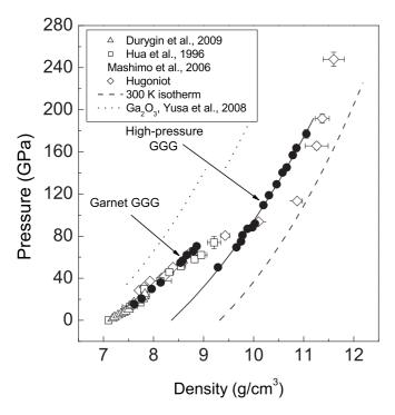
FIG. 4. Comparison of the density-pressure relationships of GGG in this study to results from Refs. 1, 9, and 11. Solid circle and line: this study; open square: from Ref. 9; open triangle: Ref. 11; open diamond: from Ref. 1; dashed line: 300 K reduced isotherm from shock-wave experiments;<sup>1</sup> dotted line:  $Ga_2O_3$  in  $Rh_2O_3$  (II) type structure and *Cmcm* structure Refs. 21 and 40.
