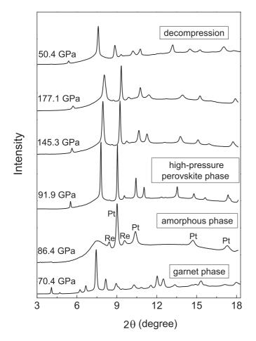
FIG. 2. Representative angle-dispersive x-ray diffraction patterns of GGG.
