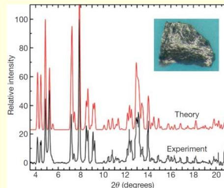
Calculated and measured XRD of  $\gamma$ -B<sub>28</sub>.
