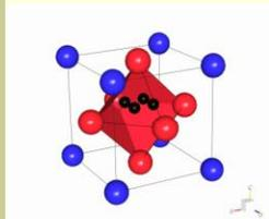
XAS shows Ti disorder in tetragonal and cubic phase → Ti displaced along {111}
