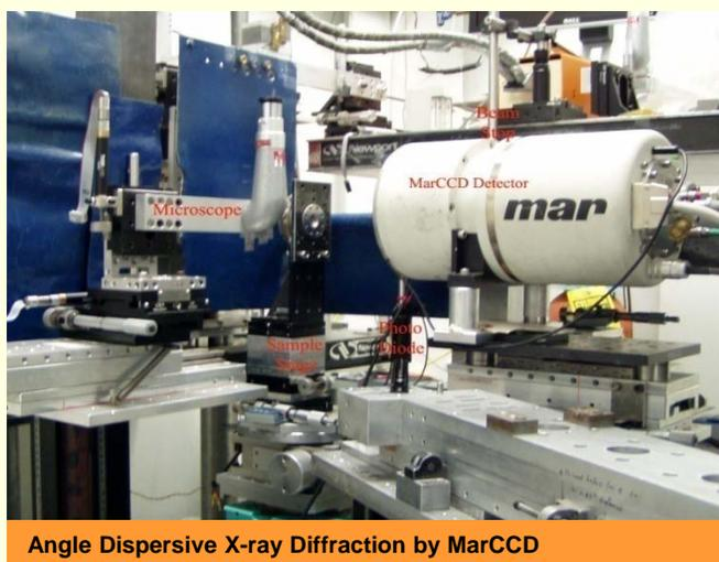
Angle Dispersive X-ray Diffraction by MarCCD
