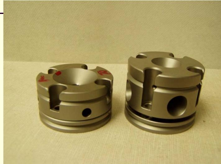
Short-Piston DAC (left) and Symmetric DAC (right)
