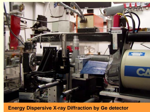
Energy Dispersive X-ray Diffraction by Ge detector
