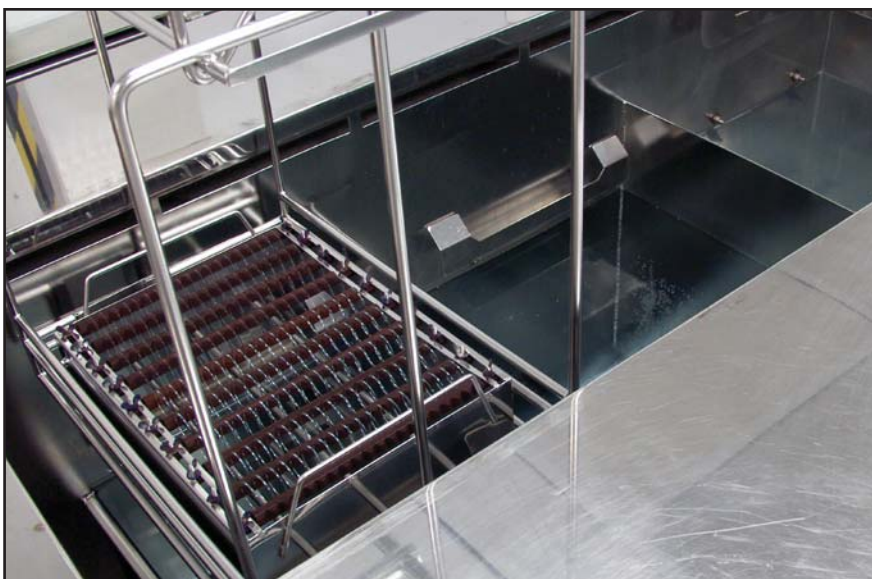
Ultrasonic cleaning is an automated multistep aqueous process for the cleaning of substrates prior to coating.
