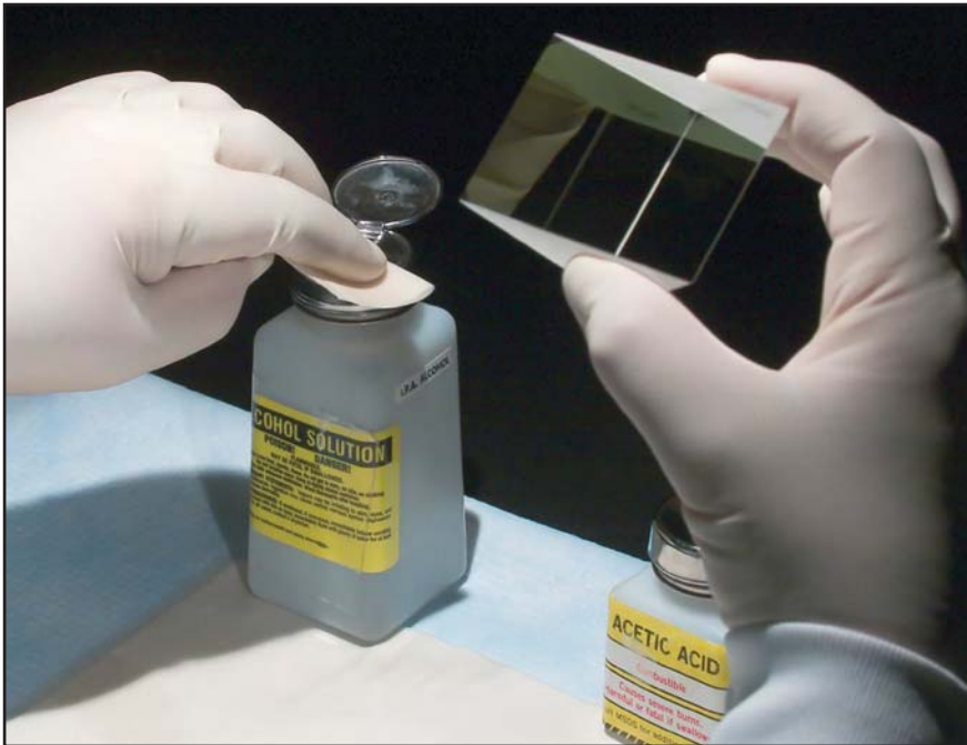
Precision optics should be handled properly in cleaning. Here, the prism is held on the frosted surfaces.
