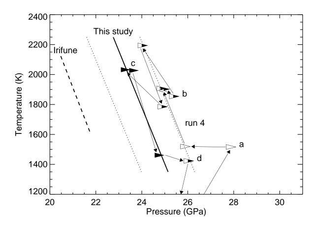
**Figure 1s.** P–T path for the run 4. This run was performed during compression. The notations for symbols follow those of figure 2 in the manuscript.
