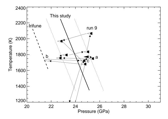
**Figure 2s.** P–T path for the run 9. This run was performed during decompression. The notations for symbols follow those of figure 2 in the manuscript.
