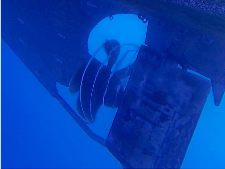
Figure 18. Cavitation generated by the propeller of the R/V Meteor during the RHUM-RUM recovery cruise. This phenomenon is due to a rapid pressure drop at the blade tips and produces high broadband acoustic noise.
