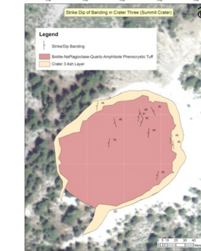
Figure 13: The Crater 3 area, derived from a satellite image, is marked in pink and the ash layer is shown in tan. The waypoints showing the strike and dip of banding is depicted to show how almost all the beds have a similar strike and dip showing that the eruption blew through pre-existing geological structures. The strike and dip measurements were also taken for banding and jointing, but these did not show any significant patterns that would have enabled us to identify any geologic units in the crater. The rotation direction of the symbol represents the strike, while the label shows the dip.
