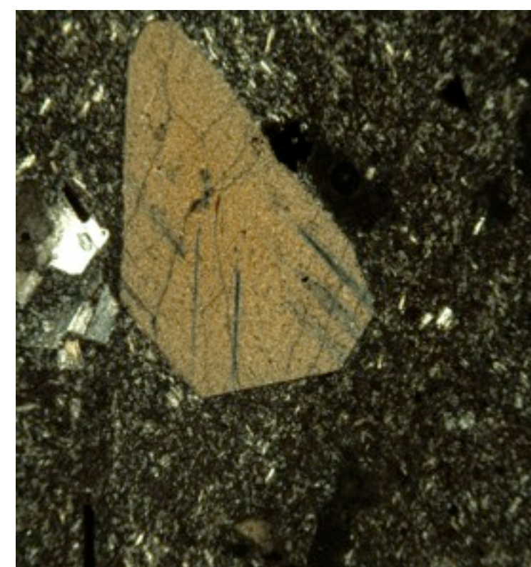
Figure 5: Photo of a thin-section of ash layer tuff from Summit Crater. Like the outcrop tuff, this tuff also contains biotite, hornblende, Na-plagioclase, quartz, and feldspar.
