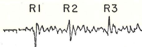
FIG. 3. Observations on a 4.46 inch diameter sphere of R_1 , R_2 , and R_3 . The phase R_3 is shifted 180^\circ with respect to R_1 because of the polar phase shifts.
