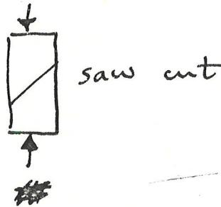
shear stress on saw cut required to cause sliding
