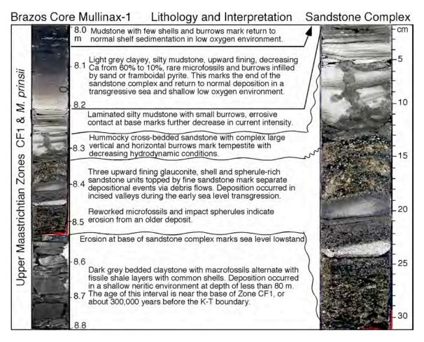
Fig. 6. Lithology, description and interpretation of the sandstone complex in core Mullinax-1. Note the three upward fining, glauconitic, spherule-rich, coarse sandstone units suggest deposition by tempestites. The overlying bioturbated hummocky cross-bedded sandstone, finely bedded sandstone and upward fining indicate decreasing hydrodynamic conditions and a return to normal shallow shelf sedimentation. Modified from Keller et al., 2007.
